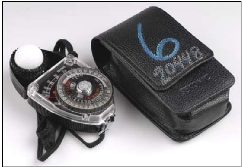
Above: The analogue light meter and case. All meters have rotating heads and protective slides for outdoor bright-light metering.
