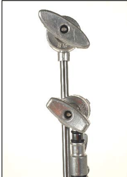
Above: Right hand rule is very important when using a C-Stand. Make sure that when you set up a C-Stand that the knuckles are to the right.
