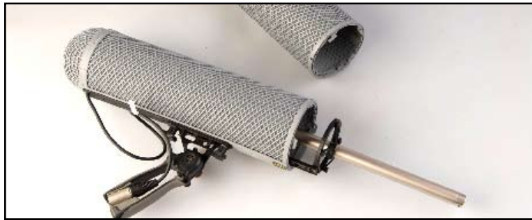
Above: The 816 with the Rycote open so you can see the microphone.
