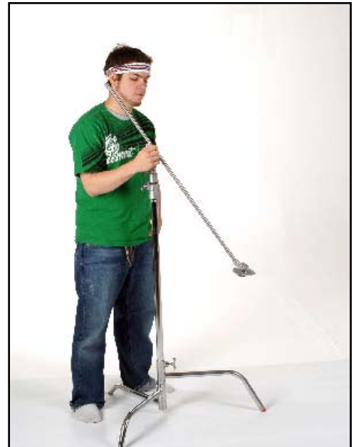
Above: Right hand rule is very important when using a C-Stand. Make sure that when you set up a C-Stand that the knuckles are to the right.
