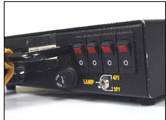
Above: The back of the Kino ballast has a switch so you can turn on or off each individual tube. It also has a lamp strength switch.
