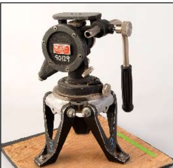
Above: High Hat three has its own head that only uses 1/4 20 screw.
