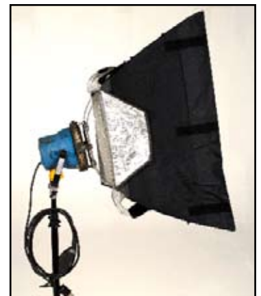
Above: The 1K with the chimera attached. Note that the flaps are left open.
