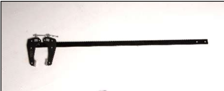
Above: The Space Clamp is a good tool to use to attach lights to beams and other objects that the C-Clamps aren't big enough to get around. However try not put a bunch of weight on them.
