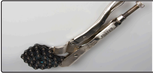
Above: Chain Vise Grip, used to clamp a small light to just about any object the chain can fit around.
