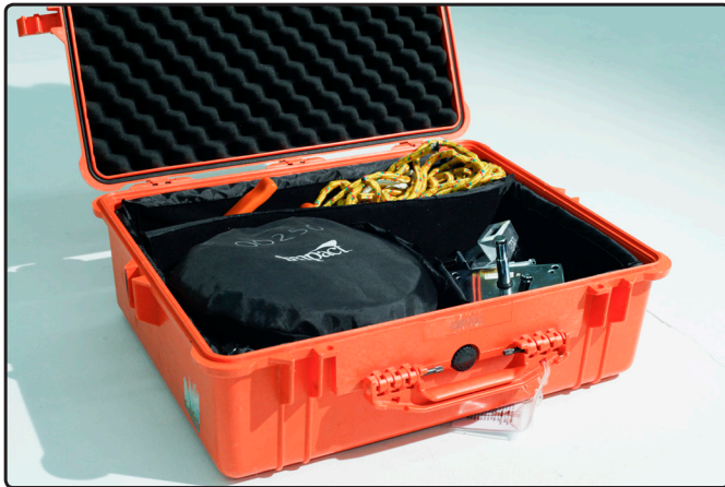
Above: All the clips and rope go in the one case, be careful with the scissor clamps, they can be bent, and if they bend too much and get broken, you have to replace them.
