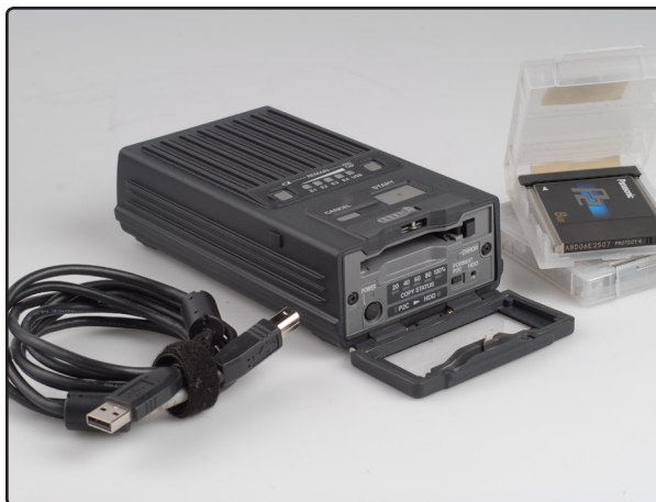
Above: The dump drive, stores up to 60GB of footage. Each of the HVX-200 HD kits come with two P2 storage cards. It must be on a stable, level surface while dumping or it may lose footage!
