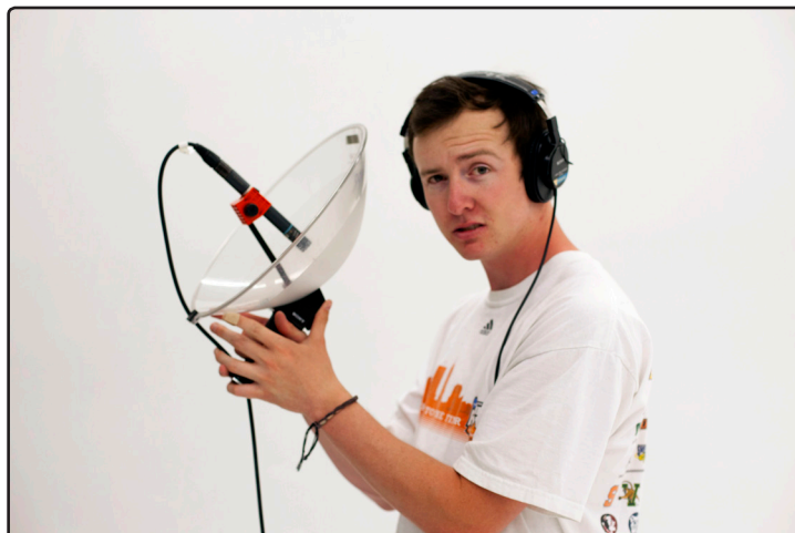
Above: The Parabolic reflector is great for spotting events and doc shoots when you are unable to get close to the action of whatever is going on.
