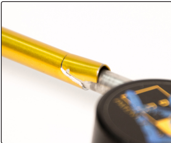
Above: The frames break easily if they are forced or not used properly. Some of the kits contain broken frames. Check the kit thoroughly when you check it out.
