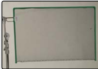
Above: 18in. x 24in. Single Net, Singles are denoted by the green fabric around the edge, a single cuts down one stop of light.
