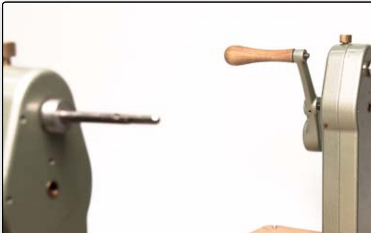
Above: The Film Rewind board is really helpful when you are trying to break a 400 foot load into daylight cores
