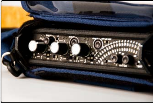
Above: Take advantage of this mixer's preamps (better quality than the cameras) and full meter L.E.D.
