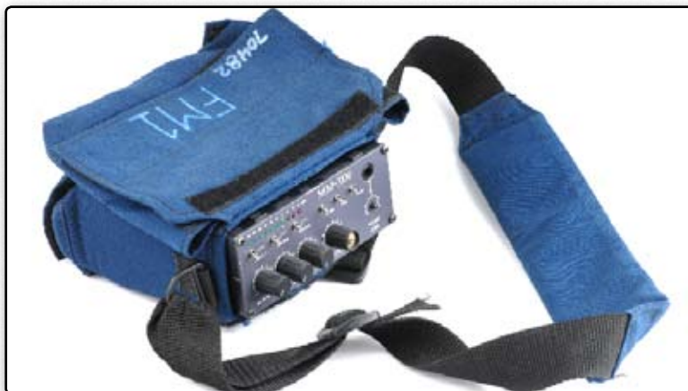
Below: If you need to mix three channels down to one this is what you should use.
