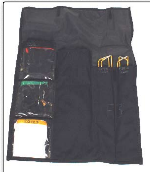
Above: The frames break easily if they are forced or not used properly. Some of the kits contain broken frames. Check the kit thoroughly when you check it out.
