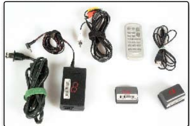
Camera accessories (from left): power cord, power adapter, RCA cable, batteries, remote, USB cable.
