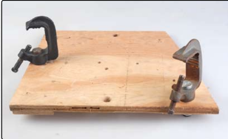
Above: C-Clamp board is used to mount a camera to the grid in Studio B
