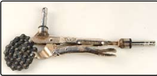
Above: Chain Vise Grip, used to clamp a small light to just about any object the chain can fit around.
