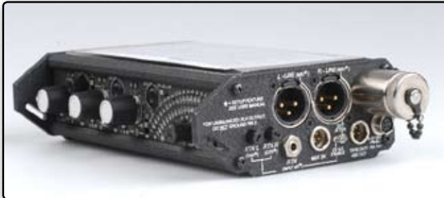
Above: The 302 has two out puts, great for running into a camera.
