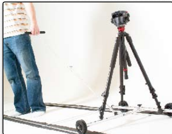
Left: the dolly set up and demonstrated with a tripod. It is intended to be pulled, not pushed.
