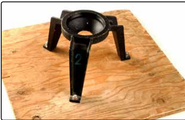
Above: High Hat two has fixed legs that will not move even if you take it off the plywood, do not remove from board.
