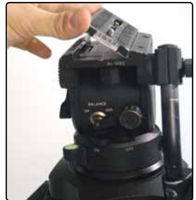
Above: This is the proper way to attach the plate to the head, it snaps down - it does not slide in!
