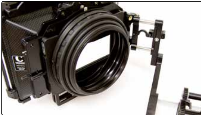
The Matte Box can be opened to make lens changing easy.
