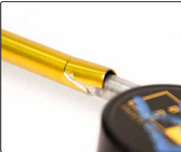
Above: The frames break easily if they are forced or not used properly. Some of the kits contain broken frames. Check the kit thoroughly when you check it out.
